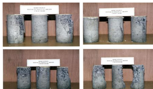
Gambar 2 Ragam keruntuhan beton
