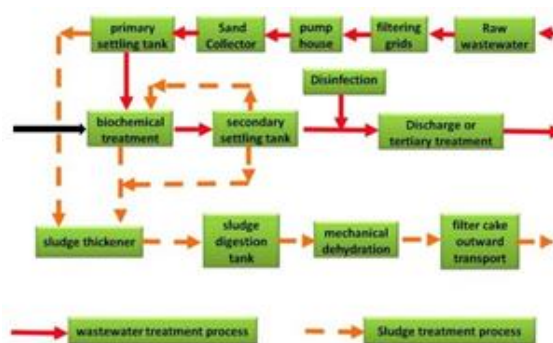
Figure 6 Flow diagram process on municipal waste water treatment
